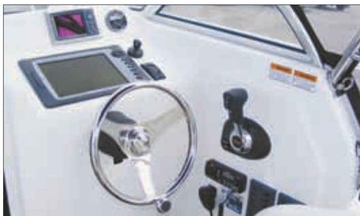
Wheel knob works well – neat dash uses only two screens rather than many gauges, fly-by-wire throttle/tilt is set beautifully to hand ...
