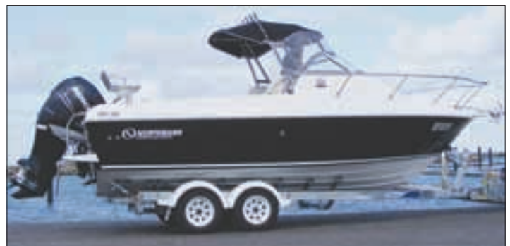
Mounted on a dual-axle Dunbier trailer fitted with Carlisle HydraStar electric hydraulic braking system for on-road safety and stability...
